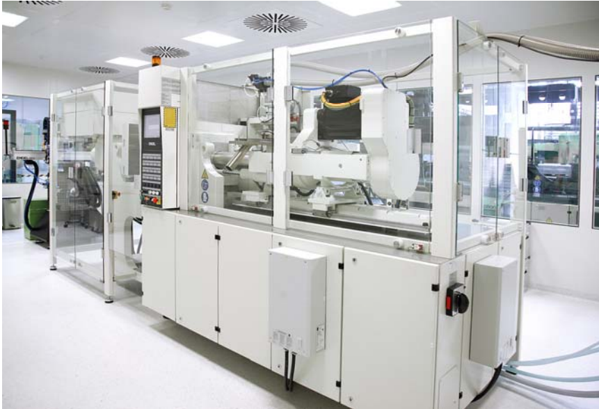
GMP-qualified ENGEL e-victory 80/50 medical injection moulding machine with a small six-axis TX40 robot by Stäubli
