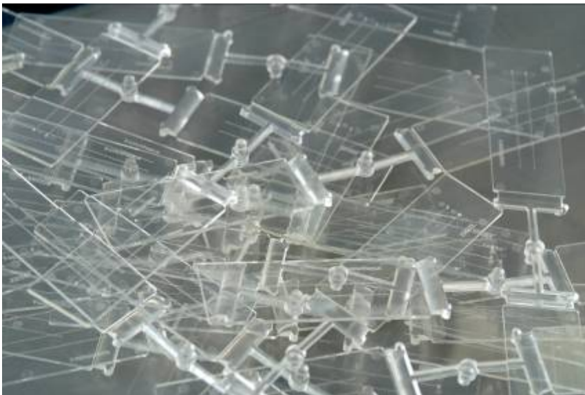
Micro-structured plastic plate with miniature channels and gutters made of Cyclo Olefin Copolymer (COC), produced in a 2-cavity mould on the new tiebar-less, and GMP-qualified ENGEL e-victory 80/50 "Medical" injection moulding machine
