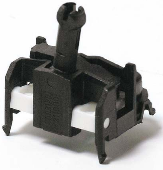
Switch made of polyamide and polyoxymethylene, produce using ENGEL's combimelt three-component technology using a 3*4-cavity ENGEL mould on an ENGEL victory 330H/80W/80V/130
