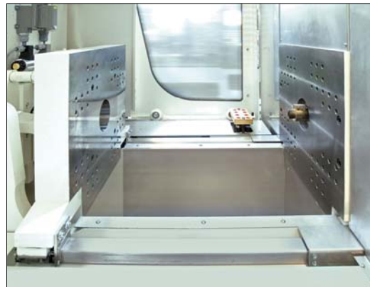
Figures 4 and 5: Tie-bar-less machine: a simple and robust concept that has been built 35,000 times. The guides of the movable plate can be displaced laterally and/or completely encapsulated, and the injection unit can be sealed off by a bulkhead.
