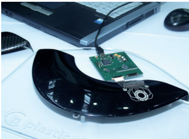
In the Clearmelt process, the substrate component is overmolded with transparent PU. In this case, a keypad with an electrical circuit is incorporated under the 0.5 mm thick overmolded layer. The keypad may be operated by gently touching the surface with a fingertip
