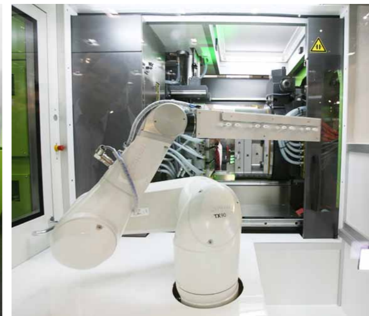
Simple integration of an industrial robot thanks to ENGEL easix: for simple and cost-effective implementation of your six-axis robot applications in medical technology. Particularly in combination with tie-bar-less injection moulding machines and filter-fan units, all benefits are combined in a compact production cell (Picture: Staubli robot TX90).
