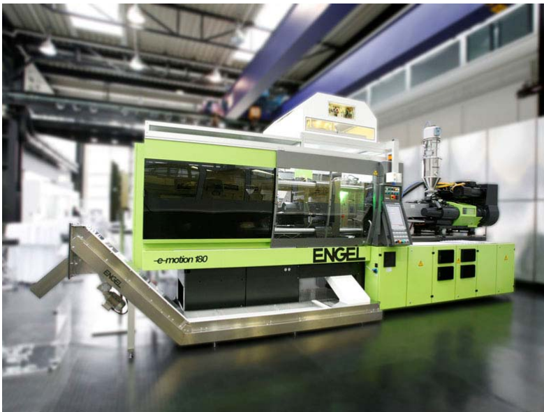
Picture 4: An ENGEL e-motion 740/180 T demonstrated the production of an innovative thin-walled syringe barrel
